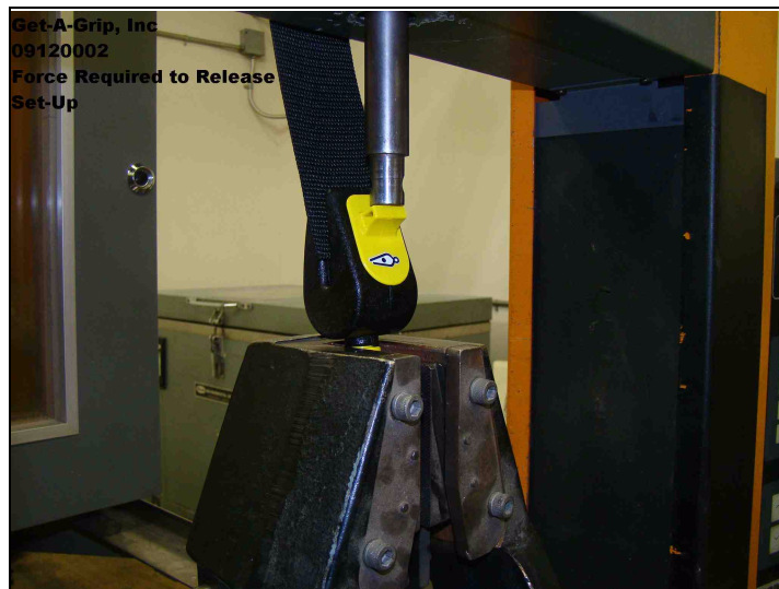
Compression Release Test (set-up photo)
